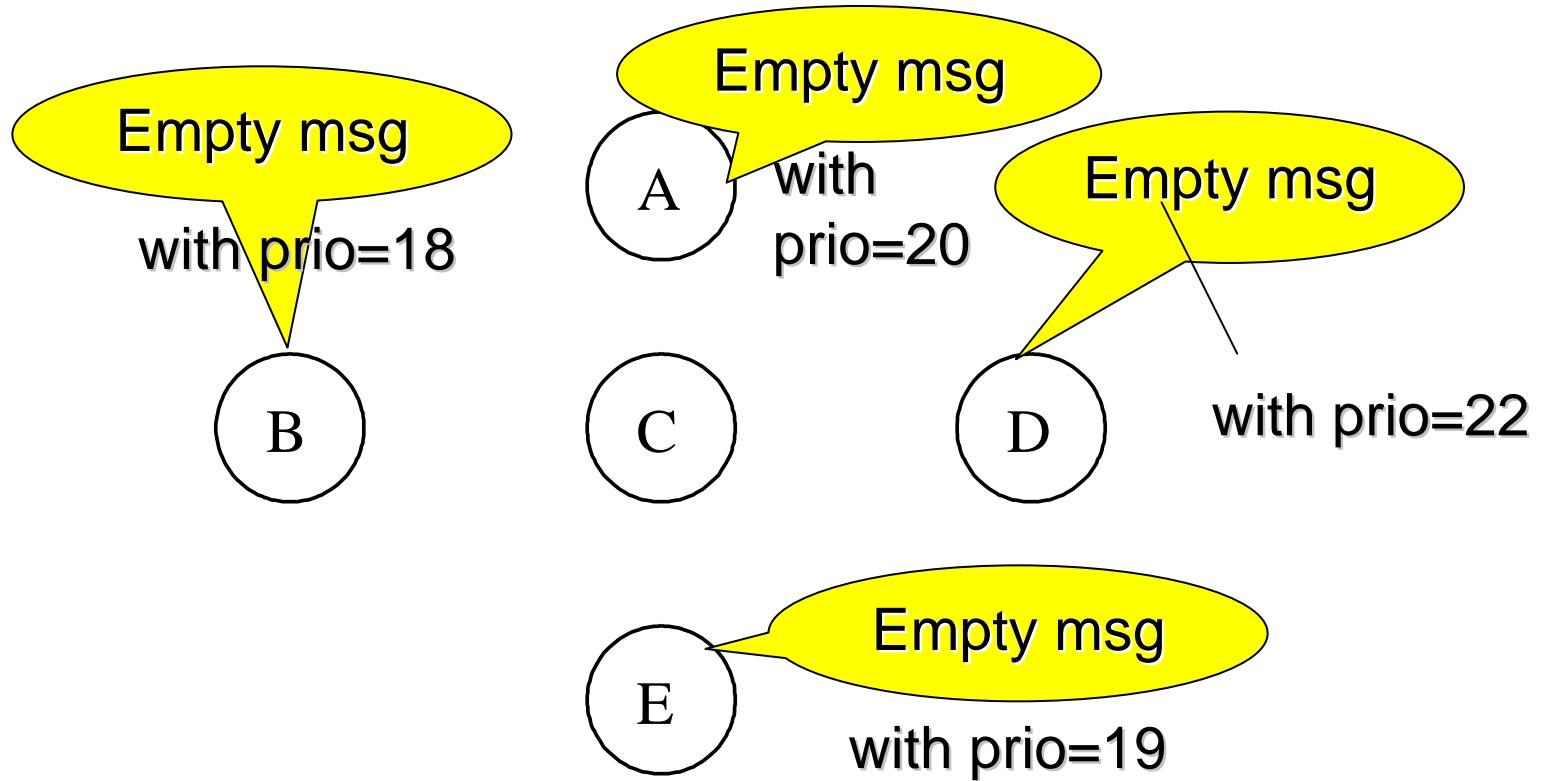
By transmitting empty msg. The priority of the msg is given by the temperature.
